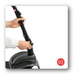
Adjusting the steering column of your scooter enables you to set the driving position so that it is comfortable.
