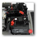
Only use batteries that are approved for this scooter (see Technical data). Ensure that the scooter is switched off before starting to replace the batteries. The batteries are located under the seat of the scooter and are protected by the housing cover.
